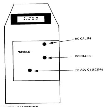
SHIELD MUST BE IN PLACE WHEN MAKING HF ADJUSTMENT.
